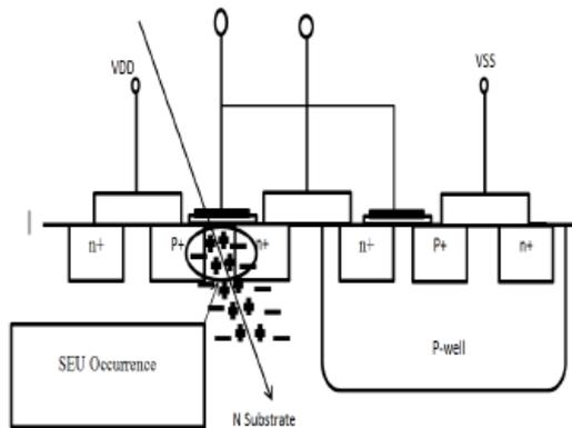
Fig. 2: SEU in CMOS memory cell
