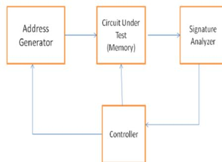
Fig.1: Architecture of Built-in-self-test
