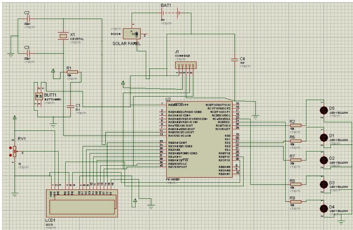
written in C Language on MPLAB IDE. After the simulation, the circuit network was designed with the help of PROTEUS ARES. After successful simulation and network design, the circuit was printed on a PCB. When the circuit printing was done on the PCB, it was drilled, and then all the components required in the system were placed manually according to the schematic of the Passenger Information Display System. Soldering of all those components was done on their respective places [10].
