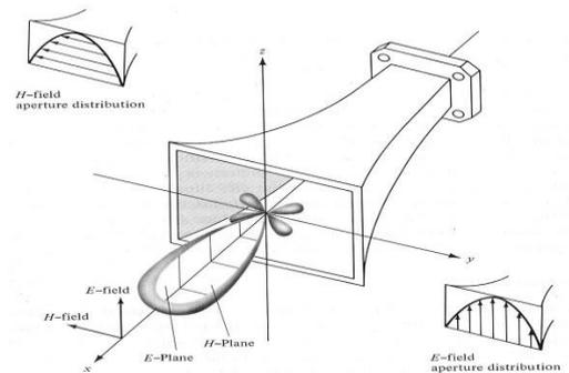
**FIGURE-3: HORN ANTENNA**
