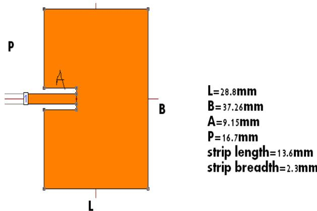
The above figure shows our receiver that was used for receiving the direct microwaves at the frequency of 2.45 Ghz. This was kept in direct touch of microwaves through which electrical pulses were produced. These pulses were fed to our rectifier circuit and we got DC voltage in millivolts. This is a metamaterial and can be improved gradually.
