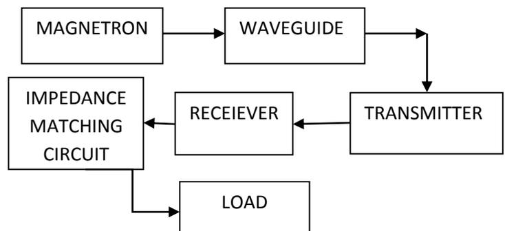
As shown above is the circuit diagram of wireless transmission of electrical energy. An oscillator i.e. magnetron is used for generating microwaves i.e. electromagnetic waves at the frequency of 2.45 Ghz. As a
