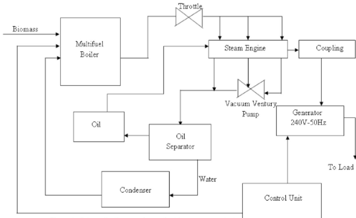
Figure 1: Schematic diagram of a captive biomass power plant
